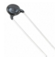
ERZ-E07A271CS Panasonic Electronic Components VARISTOR 270V 2.5KA DISC 9MM
