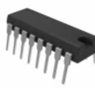
MM74HC165N Fairchild/ON Semiconductor IC REGIST PAR-IN/SER-OUT 16-DIP
