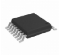
MM74HC165MTCX Fairchild/ON Semiconductor IC SHIFT REG 8BIT PISO 16-TSSOP
