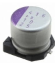
25SVPD10M Panasonic Electronic Components CAP ALUM POLY 10UF 20% 25V SMD
