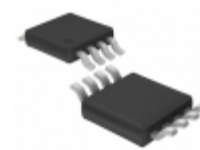
LTC1550LCMS8-2#TRPBF ADI (Analog Devices, Inc.) IC REG SWTCHD CAP INV -2V 8MSOP
