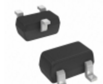
DDTA115GE-7-F Diodes Incorporated TRANS PREBIAS PNP 150MW SOT523
