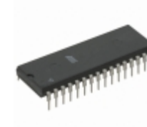
AT28C010-12PC Microchip Technology IC EEPROM 1MBIT 120NS 32DIP
