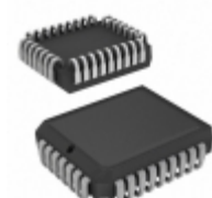
AT28C010-12JA Microchip Technology IC EEPROM 1MBIT 120NS 32PLCC
