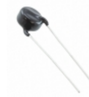
ERZ-E08A621 Panasonic Electronic Components VARISTOR 620V 3.5KA DISC 11.5MM
