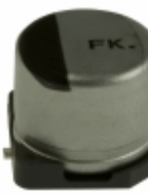
EEE-FK1E101XP Panasonic Electronic Components CAP ALUM 100UF 20% 25V SMD
