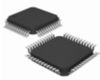
CPC7601KTR IXYS Integrated Circuits Division IC ANALOG SWITCH 16CH 48-LQFP
