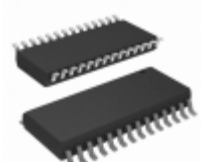
CPC7695BBTR IXYS Integrated Circuits Division IC LINE CARD ACCESS SW 28-SOIC
