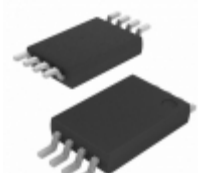
BR24S32FVT-WE2 Rohm Semiconductor IC EEPROM 32KBIT 400KHZ 8TSSOP-B
