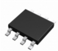
BR24S32FVM-WTR Rohm Semiconductor IC EEPROM 32KBIT 400KHZ 8MSOP
