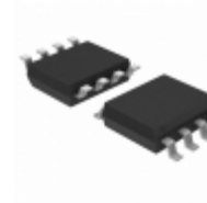
24LC08BT-I/SN Microchip Technology IC EEPROM 8KBIT 400KHZ 8SOIC
