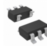
24LC08BT-I/OT Microchip Technology IC EEPROM 8KBIT 400KHZ SOT23-5
