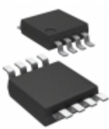
24LC08BT-I/MS Microchip Technology IC EEPROM 8KBIT 400KHZ 8MSOP
