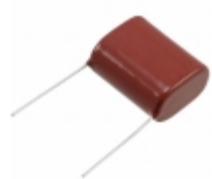
ECQ-E2106KF Panasonic Electronic Components CAP FILM 10UF 10% 250VDC RADIAL
