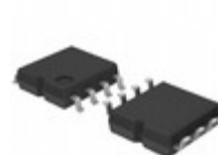
BR93G86F-3BGTE2 LAPIS Semiconductor MICROWIRE BUS 16KBIT(1024X16BIT)
