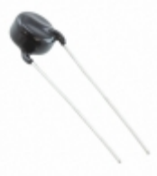
ERZ-E08A681 Panasonic Electronic Components VARISTOR 680V 3.5KA DISC 11.5MM
