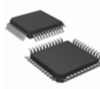
TS87C58X2-MCC Microchip Technology IC MCU 8BIT 32KB OTP 44QFP
