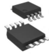
DS1135LU-20+T&R Maxim Integrated IC DELAY LINE 20NS 8UMAX
