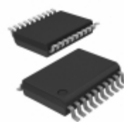
PIC16C770T-I/SS Microchip Technology IC MCU 8BIT 3.5KB OTP 20SSOP
