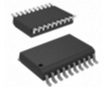
PIC16C770T/SO Microchip Technology IC MCU 8BIT 3.5KB OTP 20SOIC
