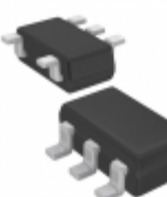
XC6121D441MR-G Torex Semiconductor Ltd IC WATCHDOG TIMER SOT-25
