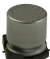
EEV-FK1C152Q Panasonic Electronic Components CAP ALUM 1500UF 20% 16V SMD
