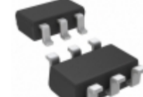
LT6700CS6-3#TRMPBF Linear Technology IC COMP DUAL 400MV REF TSOT23-6
