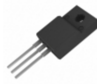
AOTF27S60L Alpha & Omega Semiconductor Inc. MOSFET N-CH 600V 27A TO220F
