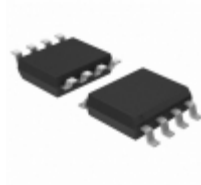
MCP3202-CI/SN Microchip Technology IC ADC 12BIT DUAL CHAN 8SOIC
