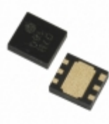
XC6122D340ER-G Torex Semiconductor Ltd IC WATCHDOG TIMER 6-USP
