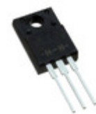
TSM7N90CI C0G TSC (Taiwan Semiconductor) MOSFET N-CHANNEL 900V 7A ITO220
