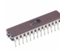
PIC14000/JW Microchip Technology IC MCU 8BIT 7KB EPROM 28CDIP
