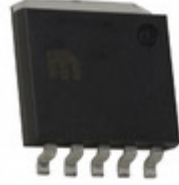
MIC37151-1.5WR-TR Microchip Technology IC REG LDO 1.5V 1.5A SPAK-5
