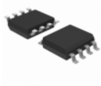
MAX7401CSA+T Maxim Integrated IC FILTER LOWPASS 8-SOIC
