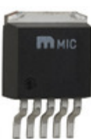
MIC39501-2.5BU Microchip Technology IC REG LDO 2.5V 5A TO263-5
