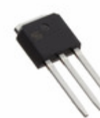
TSM60NB380CH C5G TSC (Taiwan Semiconductor) MOSFET N-CH 600V 9.5A TO251
