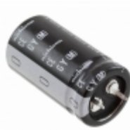
LGY2Z561MELZ Nichicon CAP ALUM 560UF 20% 180V SNAP
