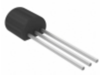
FJN3301RBU AMI Semiconductor / ON Semiconductor TRANS NPN 50V 0.1A TO-92
