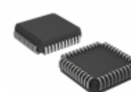
AT89S8253-24JU Microchip Technology IC MCU 8BIT 12KB FLASH 44PLCC
