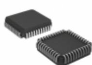
AT89S8253-24JC Microchip Technology IC MCU 8BIT 12KB FLASH 44PLCC
