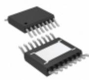
LT8610ACIMSE#PBF Linear Technology IC REG BUCK ADJ 3.5A SYNC 16MSOP
