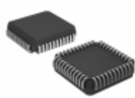
ISPLSI 1016EA-200LJ44 Lattice Semiconductor Corporation IC CPLD 64MC 4.5NS 44PLCC
