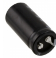
LGN2C102MELZ45 Nichicon CAP ALUM 1000UF 20% 160V SNAP
