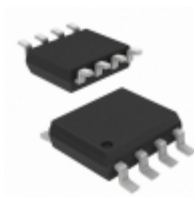
IRF7241 Infineon Technologies MOSFET P-CH 40V 6.2A 8-SOIC
