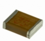
MC18FD151G-F Cornell Dubilier Electronics (CDE) CAP MICA 150PF 2% 500V 1812
