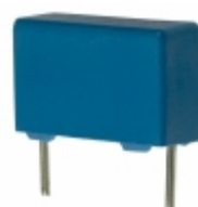
B32522C6154J EPCOS (TDK) CAP FILM 0.15UF 5% 400VDC RADIAL
