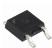
FDD6796A Fairchild/ON Semiconductor MOSFET NCH 25V 20A DPAK
