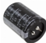
LGY2E102MELC Nichicon CAP ALUM 1000UF 20% 250V SNAP
