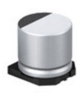
EEE-FK1C432SM Panasonic CAP ALUM 4300UF 20% 16V SMD
