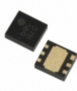
XC6121A748ER-G Torex Semiconductor Ltd IC WATCHDOG TIMER 6-USP
