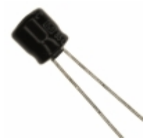
ECE-A1CKs220I Panasonic Electronic Components CAP ALUM 22UF 20% 16V RADIAL
