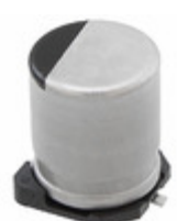
EEE-FT1E471GP Panasonic Electronic Components CAP ALUM 470UF 20% 25V SMD
