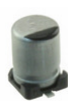
EEE-FT1E220AR Panasonic Electronic Components CAP ALUM 22UF 20% 25V SMD
