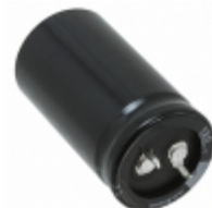
LGR2G181MELA45 Nichicon CAP ALUM 180UF 20% 400V SNAP
