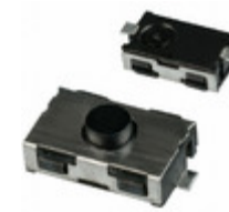
KSR221G C&K SWITCH TACTILE SPST-NO 0.05A 32V
