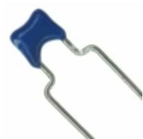
B37987F1223K000 EPCOS (TDK) CAP CER 0.022UF 100V X7R RADIAL
