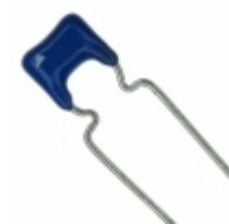
B37987F1104K000 EPCOS (TDK) CAP CER 0.1UF 100V X7R RADIAL
