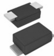
SE10FJHM3/I Electro-Films (EFI) / Vishay DIODE GEN PURP 600V 1A DO219AB
