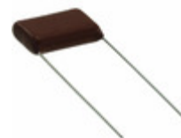
ECQ-E6104JF3 Panasonic Electronic Components CAP FILM 0.1UF 5% 630VDC RADIAL
