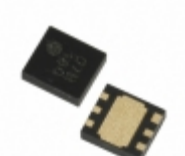
XC6123C521ER-G Torex Semiconductor Ltd IC WATCHDOG TIMER 6-USP
